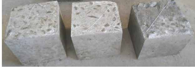
Figure 9. Rice husk ash specimens after immersing them in acid for 90 days
