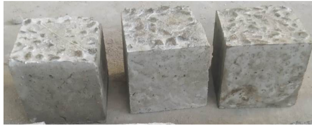
Figure 10. PET powder specimens after immersion in acid for 90 days
