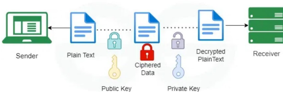
Fig-4 Mechanism of Asymmetric Key Cryptography.
