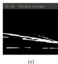
(c) Binarization shows the defects
