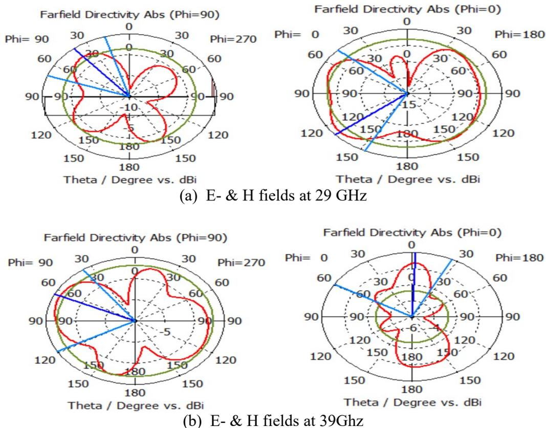
**Fig. 4.** Two-element MIMO design 2-D radiation patterns at 29 GHz and 39 GHz
