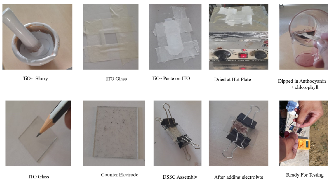
Figure 2: Dye Sensitized Solar Cell (DSSCs) Assembly
