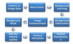
1. Camera or Image Data Acquisition1he first stage of the system is acquiring input data from a camera or pre-recorded video feed. This data acts as the primary input for vehicle detection. The camera captures continuous frames of the road or traffic, which will be processed for detecting and classifying vehicles. The system supports both live video streams and stored video files for offline processing.
