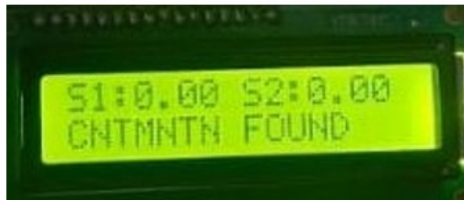
Fig. 9. message on LCD after the leakage and contamination found
