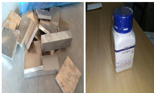
Figure 2.1 Al 5083 Matrix material and Cerium Oxide (CeO 2 ) Reinforcement material
