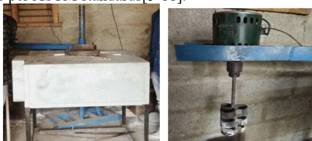
Figure 2.2 - Electrical Induction Furnace and Stirrer
