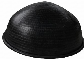
FIGURE 1. Hemispherical Aluminum absorber dome with solar-selective black coating
