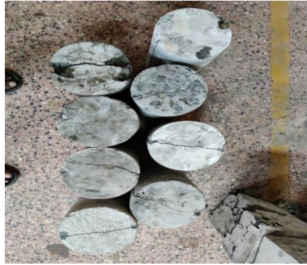
Failed cylinders after testing
