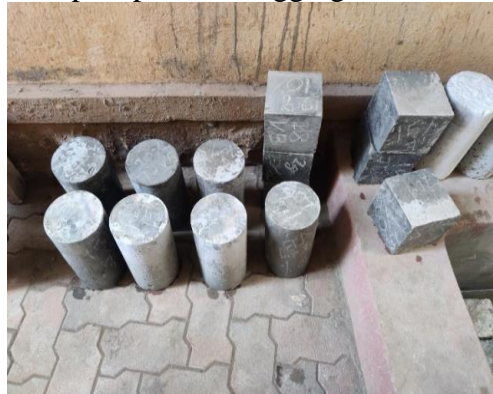
Prepared moulds of concrete mix with partial replacement
