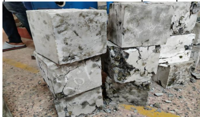
Failed cubes after testing
