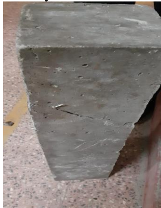
Failed beam after testing
