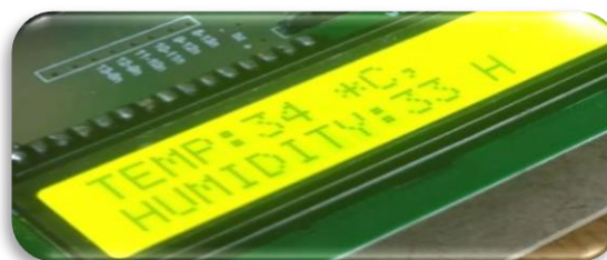
Fig 26: Temperature and Humidity values in Hot condition
