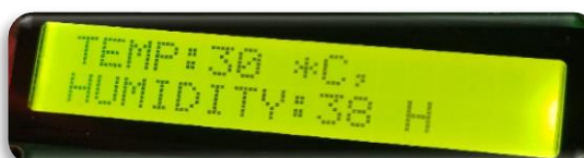
Fig 20: Temperature and Humidity values in normal condition
