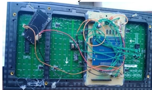
Fig.4. Circuit Board of E-Notice Board
