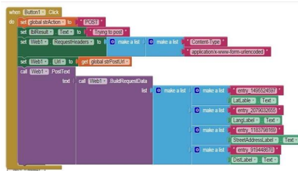
Fig. 3. Blocks for getting mobile device values and to post in Google Spreadsheet
