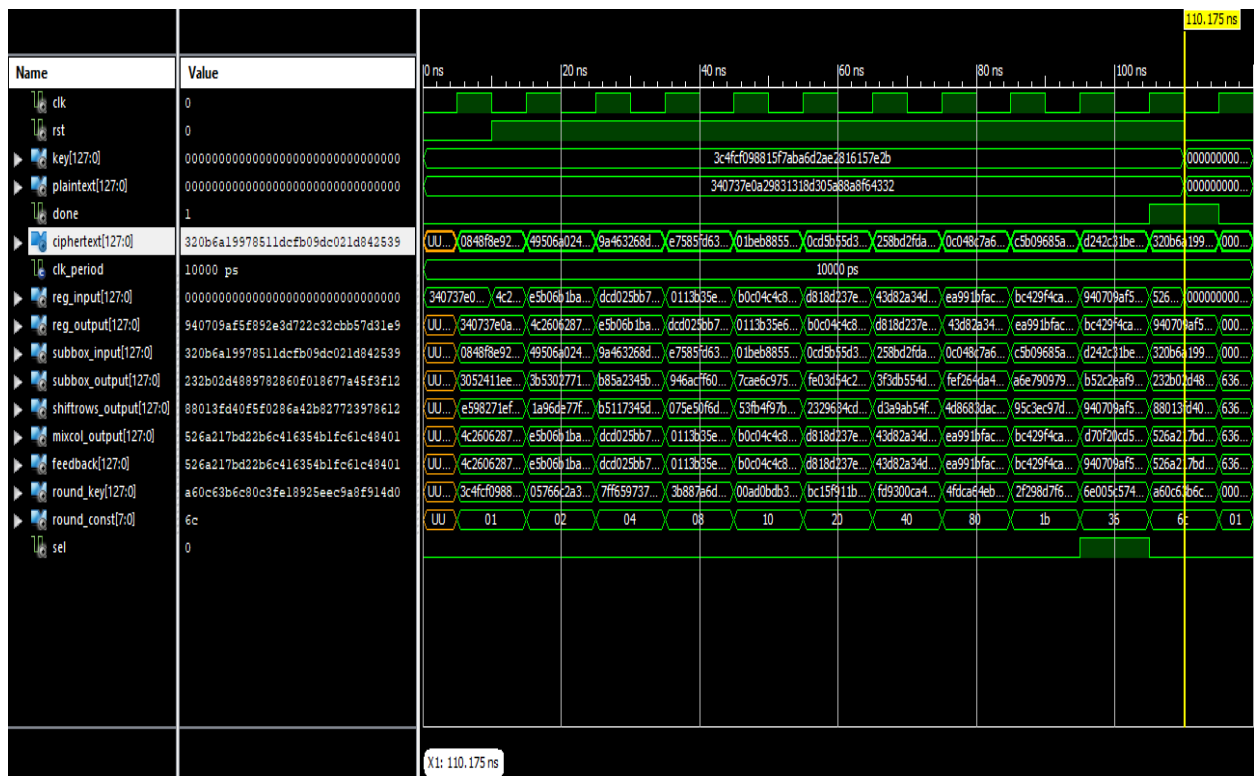
Figure 16. Test Bench wave form of AES_ENC
