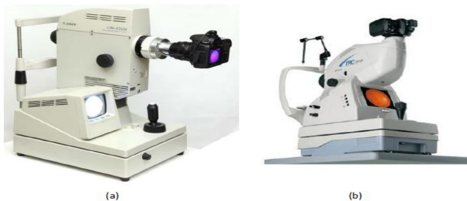
Figure 3: Two types of non-mydriatic retinal image cameras: (a) Canon CR6-45NM and (b) Topcon TRC-NW6S
