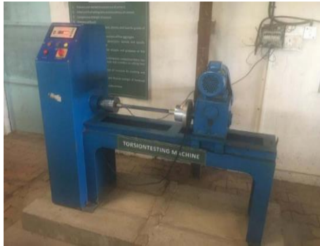
Fig. No. 7. Torsion testing machine
