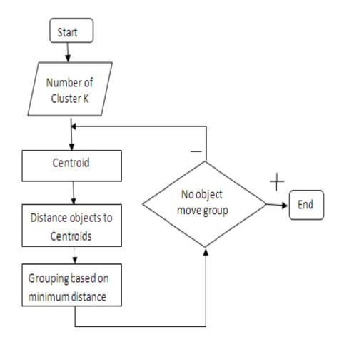
We propose an enhanced version of the k-means algorithm with simple partitioning to speed up the time in finding the final converged centroids. The pseudo-code of our algorithm. Table 1 shows the notation used in describing the algorithm. Our algorithm is composed of three parts.
