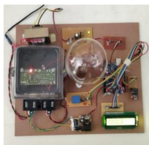
Fig 2: Smart Energy Meter Using IoT When No Load
