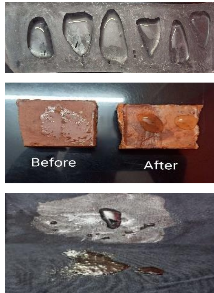
Fig. 3 : Nano self cleaning with nano materials before & after the process
