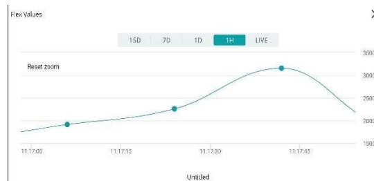
Figure: 4 Output shown on the Arduino IoTCloud application by the Flex Sensor
