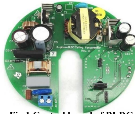
Fig.1. Control board of BLDC
