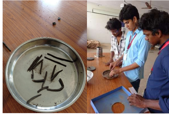
Fig 4 Plastic limit test of the soil
