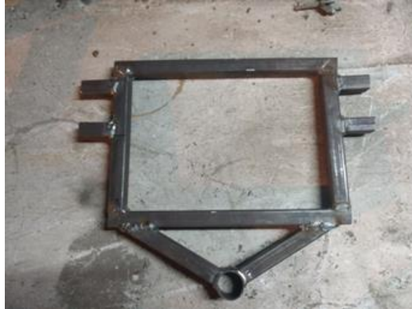
Fig. 2. Welded AISI 1020 frame before assembly.
