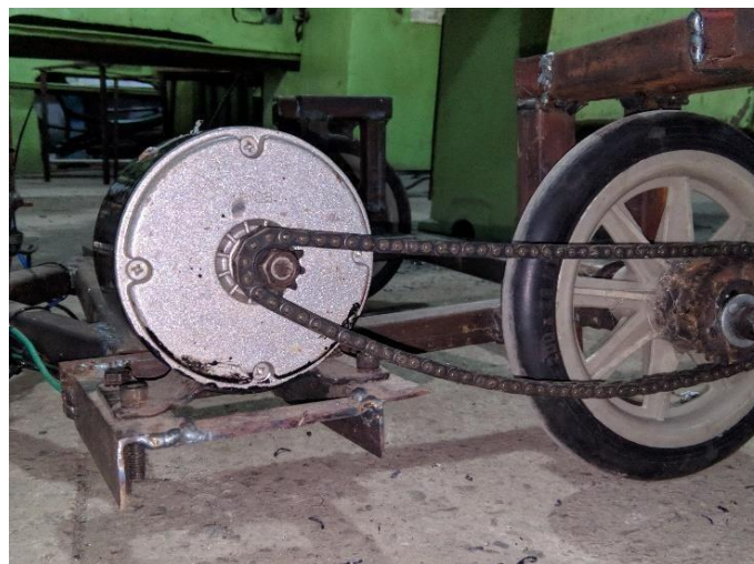
Fig. 5. Brushless DC traction motor, 250 W, 24 V.
