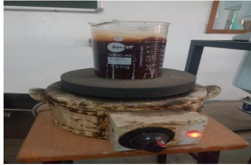
Fig.5 Continuously stirred at 90°C for 4hrs
