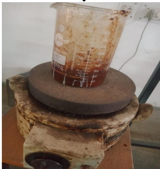
Fig.6 Removal of lignin
