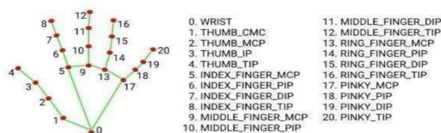
Fig. 1. Twenty-one hand landmark points defined by the MediaPipe hand tracking model.
