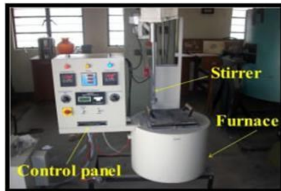
FIGURE 2.2 Components stir casting process
