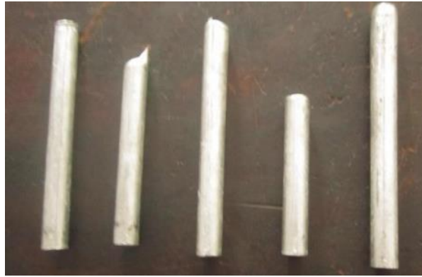
FIGURE 2.3.1 Different weight fractions of TiB 2 reinforced MMC's
