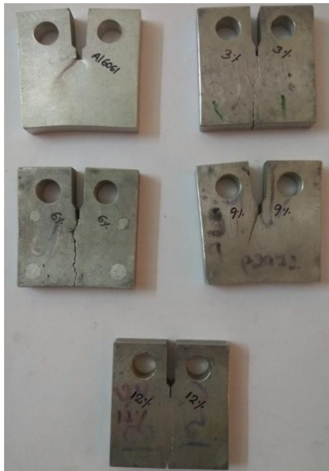
FIGURE 3.1.2 Fractured specimens of Al6061 and TiB 2 Reinforced (Base, 3%, 6%, 9% and 12%) composites.
