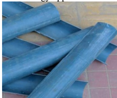
FIGURE 3. Design of Wind Turbine Blades With PVC Pipes
