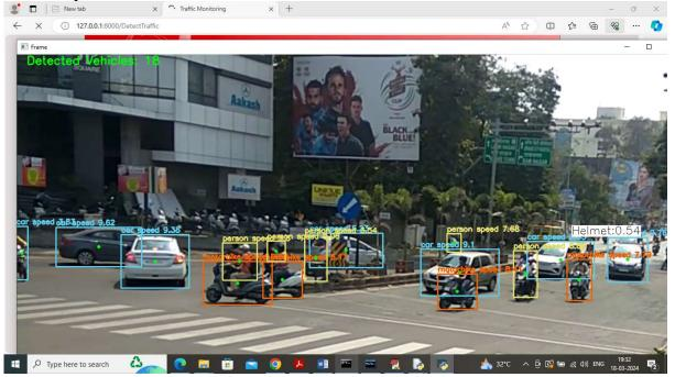
In above screen can see classify vehicles as Car, motor bike and can see Helmet class also in white colour text and in top in green colour text can number of detected traffic vehicles
